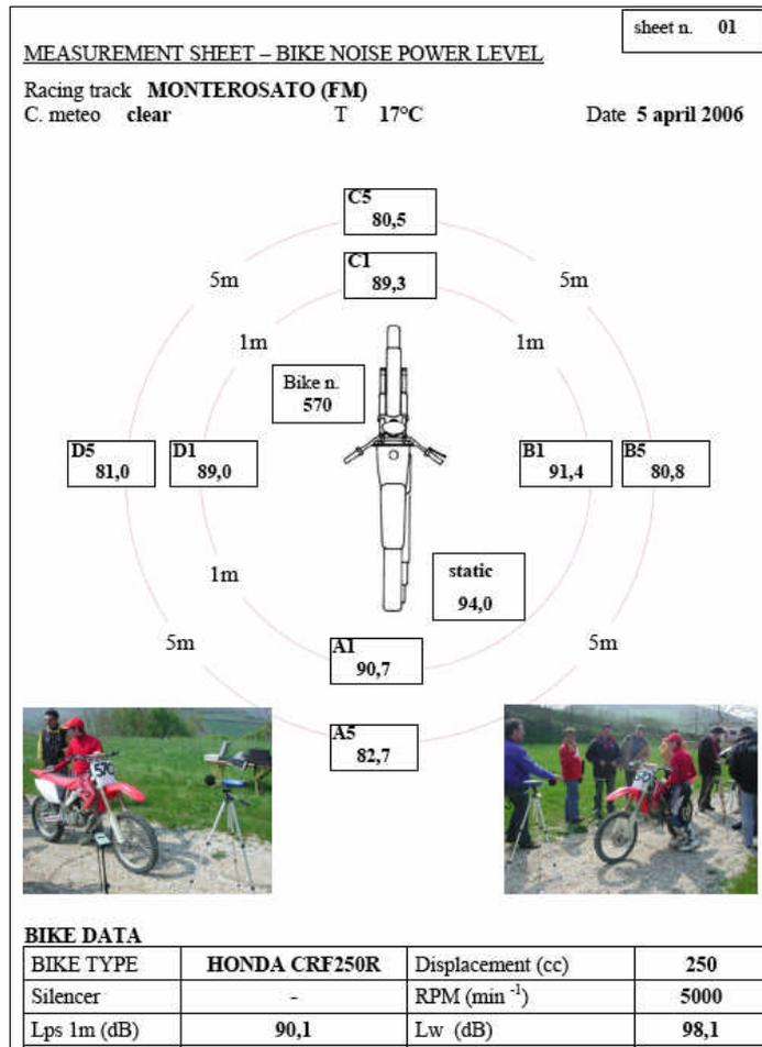
Figure 2: Noise propagation characterization.
