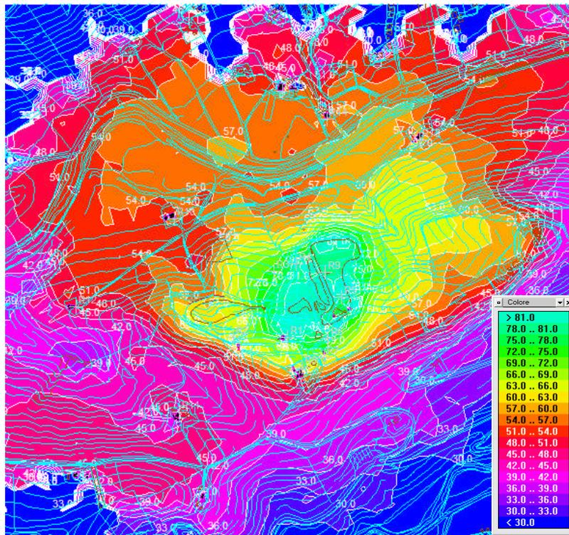
Figure 7: B group horizontal noise propagation.
