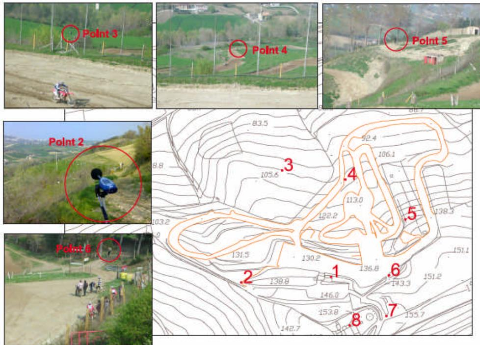
Figure 5: Noise measurement positions.
