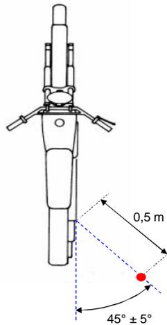
Figure 1: Static noise test method.
